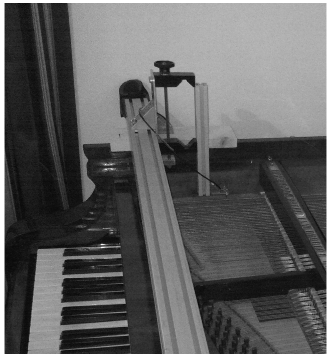
FIG. 10. Experimental setup. The string velocity is measured with an electromagnetic transducer placed near the string. The string-sensor distance is adjusted with a micrometer screw. The sensor and the screw-holder can slide from string to string along a metallic bar.
