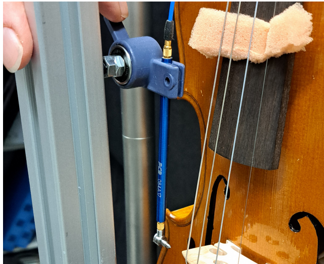
Figure 1: The PCB© impact hammer (Model 086E80 [4], aluminum handle assembly attached) is mounted as a pendulum using a custom-made 3D-printed lever and bearing device.
