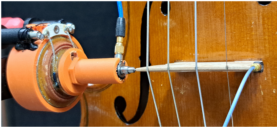
Figure 7: Excitation of a violin, using a 34 mm diameter vibration speaker (e.g. [5]) as driver. A 3D-printed centerpiece is glued on the plastic rim of the moving coil assembly to transfer the movement to the impact hammer. The shaker's small diameter allows it to fit in front of the violin body without making contact.
