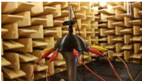
FIG. 1. (Color online) 3D-printed spherical cap with microphone for pressure gain measurements in closed state.
