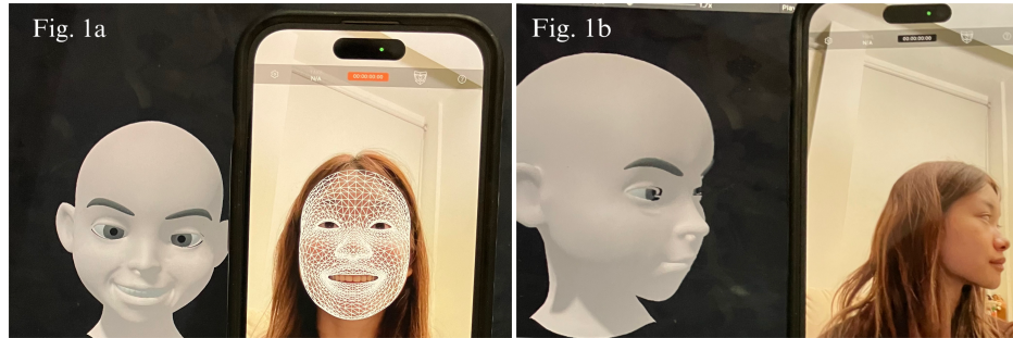
Fig. 1. A demonstration of the system specification. Using two devices, the first one being a phone with camera running Face Capture, the second one is the laptop running the Unity project. The system could be used with or without wireframes on the user's face. Fig. 1a displays the real-time reflection of the user's front profile on the avatar. Fig. 1b shows the avatar mirroring the user's head turning to the side.
